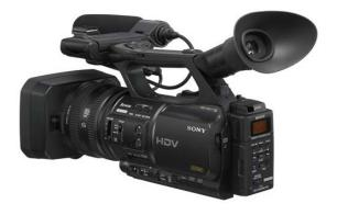
shooters. The most significant are dual XLR audio, native progressive 24p/30p, DVCAM recording, SMPTE timecode support, and full docking ability with Sony's new HVR-MRC1K compact flash recorder.
